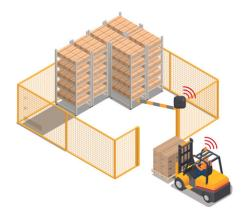
The vehicle's speed in the speed-limited zone is determined as a maximum of 10 km/h inside the warehouse. It has been installed in 19 forklifts at the moment.
